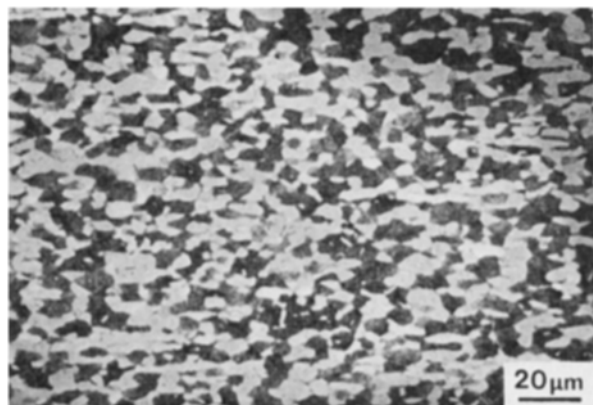
Figure 8 As Fig. 1, followed by superplastic tensile testing at 915° C to \sim 100\% strain. Longitudinal section showing coarsening of the \alpha + \beta microstructure ( D_z = 2.8 \mu\text{m} ).
